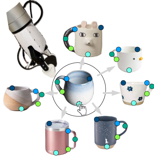
Fig. 1: A human prescribes key points one time for one instance of an object and those points are transferable to all other instances of the same object.
